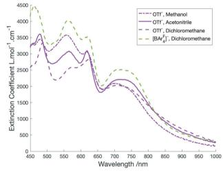
Fig. 4 Top: electronic spectra of  $[Co(dipyvd)_2]^+$  (blue), The low spin (S = 1/2) and high spin (S = 3/2) forms of  $[Co(dipyvd)_2]^{2+}$  obtained by deconvolution (yellow and orange respectively), and  $[Co(dipyvd)_2]^{3+}$ . Bottom: solvent and counterion dependence of the electronic spectrum of  $[Co(dipyvd)_2]^{2+}$ .
