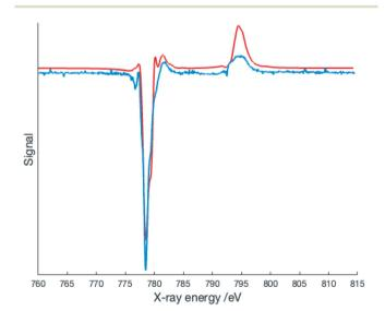
Fig. 6 XMCD spectrum of  $[Co(dipyvd)_2]^{2+}(PF_6)_2$  at 2 K/6T (blue) along with crystal field multiplet simulation (red line) – simulation parameters 10Dq = 2.0 eV, Slater–Condon integrals scaled by a factor of 0.69.
