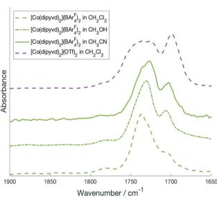
Fig. 1 Top: carbonyl region of the IR spectrum of crystalline [Co  $(dipyvd)_2$ ]<sup>2+</sup> salts. Bottom: carbonyl region of  $[Co(dipyvd)_2]^{2+}(BAr^F_4)_2$  and  $[Co(dipyvd)_2]^{2+}(OTf)_2$  in solution.
