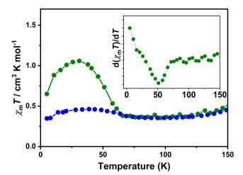
Fig. 5 Temperature-dependent magnetic susceptibilities of complex 2·0.5EtOH after irradiation (green). Light-induced magnetization is performed by 532 nm irradiation. Magnetization of the bulk sample is shown in blue circles. Inset: First-order derivatives of the light induced  $\chi_m T$  product.
