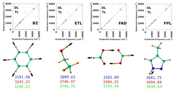
Fig. 9 Prediction of vibrational normal modes using DL and TL models of BZ, ETL, FAD, and FPL. The top panel shows scatter plots of reference-vs.predicted frequencies, while the bottom panel shows the highest frequency normal modes. The blue, red, and green numbers are respectively the reference (exact), DL, and TL predicted frequencies. The collective movements of each mode are also depicted.
