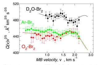
**Fig. 12** Integral cross-sections Q(v) for  $D_2O$ ,  $O_2$ , and Ar projectiles colliding at selected velocity v with  $Br_2$  targets. Data are plotted as  $Q(v) \cdot v^{2/5}$  to emphasize the glory patterns, the shifting in the extreme position and the increase in the absolute value of cross-sections.
