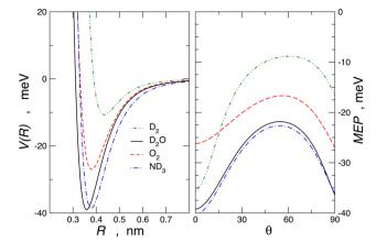
Fig. 11 Left panel: spherically averaged potential energy curves, V(R), vs. centre of mass separation distance, R, for the molecule-Br2 complexes. Right panel: minimum energy path, MEP, vs. the angular variable  $\theta$  for the Br<sub>2</sub> complexes under investigation obtained by the present potential formulation.
