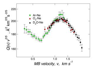
Fig. 2 Total integral cross-sections Q(v) for collisions between Ar (green),  $O_2$  (red) and  $D_2O$  (black) and Ne measured at selected beam velocity v. As usual,  $^{41-43,58}$  data are plotted as  $Q(v) \cdot v^{2/5}$  to emphasize the glory patterns. Reproduced from ref. 25 with permission from American Chemical Society, copyright © 2012.
