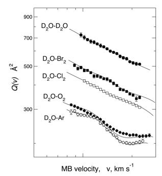
Fig. 13 Comparison of the integral cross-sections Q(v) measured, under the same experimental conditions, for the scattering of  $D_2O$  molecular beams, velocity selected in the v range, by  $Br_2$ ,  $Cl_2$  and other selected targets.
