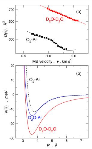
Fig. 6 Panel (a): comparison of the measured Q(v) data. Panel (b): the best fit experimental interaction potential for O2-Ar (black dashed, van der Waals), D<sub>2</sub>O-Ar (blue continuous, weak HB) and D<sub>2</sub>O-D<sub>2</sub>O (red, strong HB): 1 meV = 0.096485 kJ mol<sup>-1</sup>. Spherically averaged potentials are plotted and used for the scattering cross-section calculation reported in
