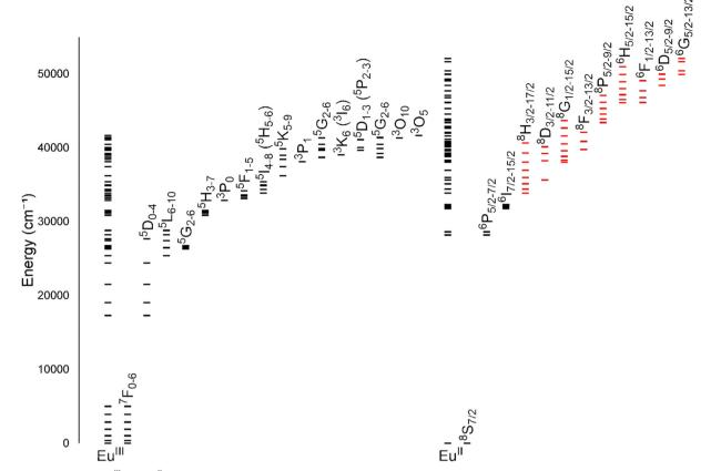
Fig. 1 Energy levels for Eu<sup>III</sup> and Eu<sup>III</sup>. All levels for each ion are shown directly over the ion label. For clarity, subsets of levels are projected to the right of the full diagram and labeled with term symbols. Projected subsets with black lines represent 4f states, and red lines represent 4f5d states. Values for the levels were obtained from previous reports. 1,2
