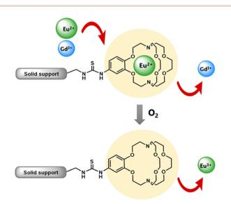
Fig. 15 Benzo-2.2.2-cryptand covalently linked to a solid support, **38**, was used to selectively separate Eu from Gd. Reprinted with permission from D. N. Kulasekara, A. B. Kajjam, S. Praneeth, T. M. Dittrich and M. J. Allen, *ACS Appl. Mater. Interfaces*, 2023, **15**, 42037. Copyright 2023 American Chemical Society.
