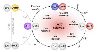
Fig. 13 Proposed catalytic mechanism of chromophore-based complexes of Eu for organic reduction reactions. Reprinted with permission from M. Tomar, R. Bhimpuria, D. Kocsi, A. Thapper and K. E. Borbas, *J. Am. Chem. Soc.*, 2023, **145**, 22555. Copyright 2023 American Chemical Society. Licensed by Creative Commons CC-BY 4.0.
