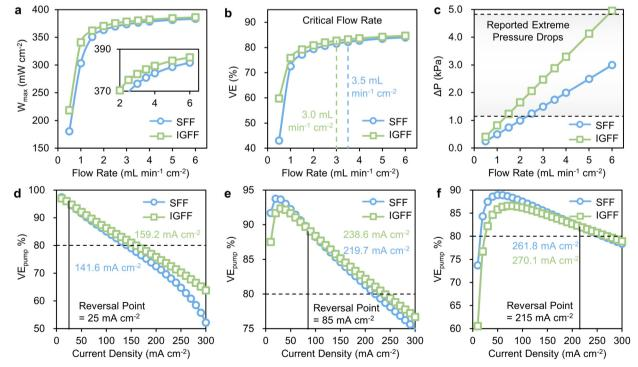
Fig. 7 The relationships of (a)  $W_{\text{max}}$ , (b) VE and (c)  $\Delta P$  with flow rates for SFF and IGFF-based VRFBs. The relationships of VE<sub>pump</sub> with current densities for SFF and IGFF-based VRFBs under flow rates at (d) 1, (e) 3 and (f) 6 mL min<sup>-1</sup> cm<sup>-2</sup>.
