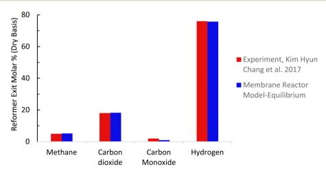
Fig. 8 Membrane reactor model validation.
