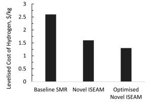
Fig. 14 Levelized cost of hydrogen comparison between baseline SMR process and novel ISEAM process at different fuel cost.
