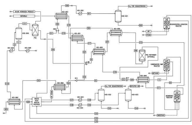
Fig. 3 Process flow diagram of a novel industrial sorption enhanced auto-thermal membrane (ISEAM) process
