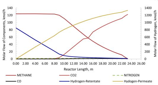
Fig. 12 Membrane reactor product profile for the novel ISEAM process (molar flow of CO<sub>2</sub>, CO, N<sub>2</sub>, H<sub>2</sub>-retentate, and H<sub>2</sub>-permeate).
