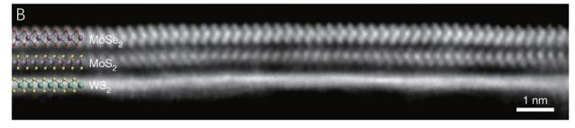
Fig. 3 (A) A schematic of the programmed vacuum stack (PVS) process. (B) The cross-sectional STEM image of a MoSe<sub>2</sub>/MoS<sub>2</sub>/WS<sub>2</sub> film with the electron beam aligned with the armchair axis of MoSe<sub>2</sub> (top) and MoS<sub>2</sub> (middle). Reproduced with permission from ref. 59, copyright Springer Nature.
