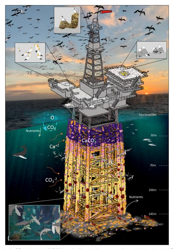
Fig. 4 Example of an OGI steel jacket in the NNS. With associated biomass in the water column from sea level through to seabed. This example has been in location for 50 years. The infrastructure is ready for the cold stage of decommissioning to commence.
