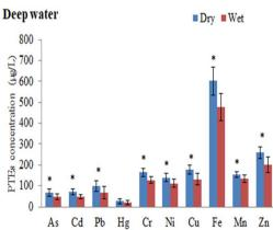
Fig. 2 Trace element concentration ( $\mu$ g L<sup>-1</sup>) in surface and deep water samples of Buriganga River in Bangladesh. "\*" indicates a statistically significant difference in TEs between the dry and wet seasons.
