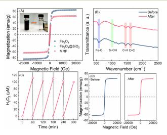
Fig. 3 (A) Magnetic hysteresis loops of the catalysts at room temperature and (A inset) magnetic separation and redispersion process of MRF; (B) FTIR spectra of MRF and reused MRF; repeated photocatalytic  $H_2O_2$  production (C) and magnetic hysteresis loops (D) of reused MRF (catalysts:  $1 \text{ g L}^{-1}$ ; pH = 7.5;  $\lambda > 420 \text{ nm}$ ; air:  $0.5 \text{ L min}^{-1}$ ).
