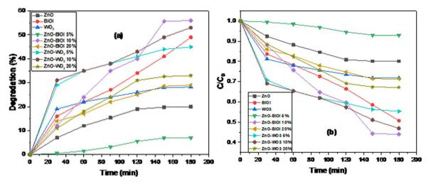
Photodegradation plots of (a) degradation efficiency, and (b) time-dependent photocatalytic degradation.
