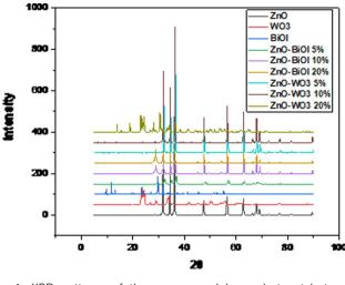
Fig. 1 XRD patterns of the as-prepared bare photocatalysts and heterostructures
