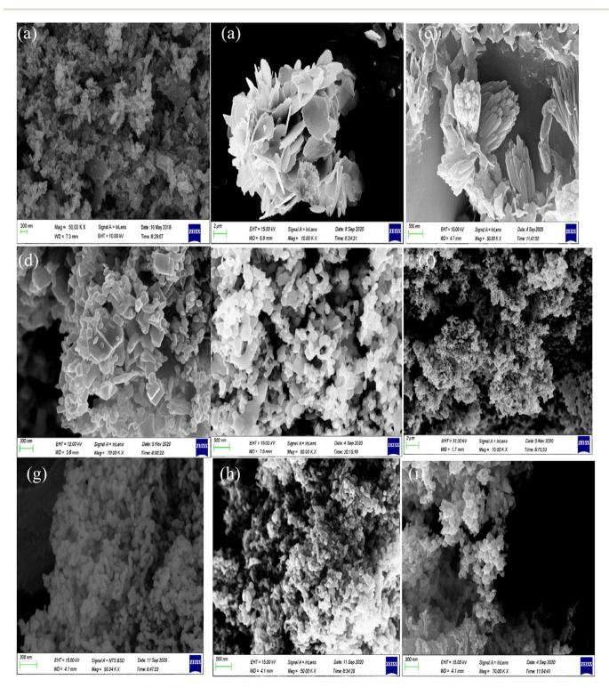
Fig. 2 SEM images of (a) ZnO, (b) BiOI, (c) WO<sub>3</sub>, (d) ZnO-[5%]BiOI, (e) ZnO-[10%]BiOI, (f) ZnO-[20%]BiOI, (g) ZnO-[5%]WO<sub>3</sub>, (h) ZnO-[10%]WO<sub>3</sub>, and (i) ZnO-[20%]WO<sub>3</sub>.
