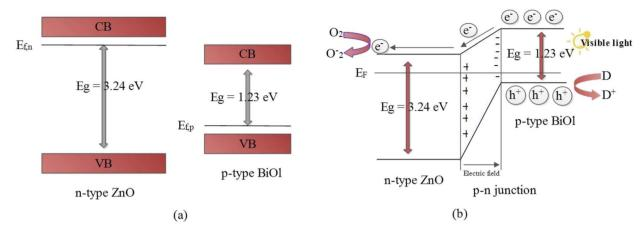
Fig. 6 Proposed band energy diagram of ZnO and BiOl before contact (a), and after (b) interfacial contact, formation of p-n junction and charge separation process of the ZnO-BiOl heterostructure under solar irradiation.
