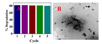
Fig. 7 Catalytic performance for 5 cycles (A) and the HRTEM micrograph (B) of the recovered AgNPs after the 5th cycle.
