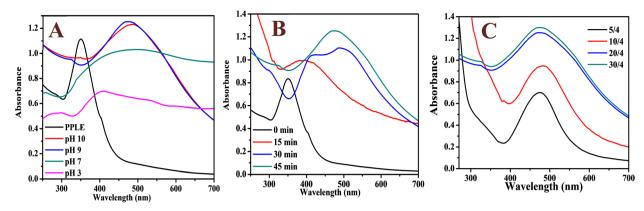
Fig. 1 UV-vis spectra of (A) the PPLE and the AgNPs synthesized at different pH, (B) time and (C) using different volumes of PPLE.
