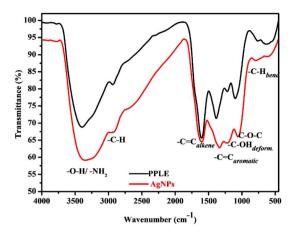
Fig. 2 FTIR spectra of the PPLE and the AgNPs.
