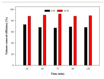
Fig. 4 Photocatalytic activity of the paint P-3 under 8 W and 24 W white light against 3 ppm toluene at a total flow rate of 50 mL min $^{-1}$ .
