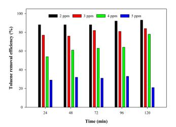
Fig. 2 Photocatalytic activity of P-1 at various toluene inputs with a total flow rate of 50 mL min<sup>-1</sup>, under 24 W white light.
