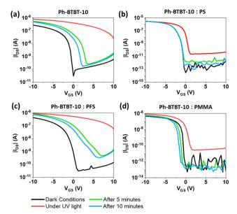
Fig. 5 Transfer characteristics curves ( $V_{DS} = -1 \text{ V}$ ) before UV exposition, under UV light and after 5 and 10 minutes of the UV light exposition for (a) pristine Ph-BTBT-10 films and Ph-BTBT-10 blend films with (b) PS, (c) PFS and (d) PMMA. The measurements were carried out under a light power of 486 µW cm<sup>-2</sup>.
