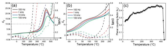
Fig. 4 (a) Temperature dependence of relative permittivity  $(\varepsilon_r)$  and loss  $(\tan \delta)$  for 0.7BiFeO<sub>3</sub>-0.3Ba $(Ti_{0.995}Nb_{0.005})O_3$  ceramics and (b) selected region illustrating variations in  $\varepsilon_r$  and  $\tan \delta$  over the temperature range from -60 to 250 °C (c) temperature-dependent planar coupling factor  $(k_p)$ .
