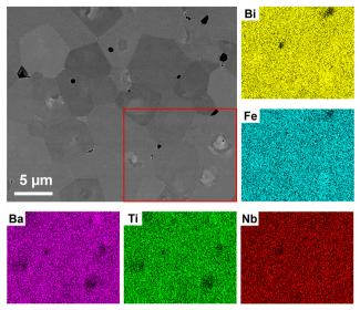
Fig. 3 SEM image (BSE mode) and EDS mapping of 0.7BiFeO<sub>3</sub>- $0.3Ba(Ti_{0.995}Nb_{0.005})O_3$  ceramic. The core regions in the red rectangular area are relatively deficient in Ba and Ti but enriched in Bi and Fe.
