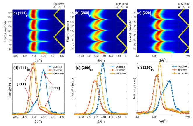
Fig. 7 Contour plots of Nb-doped 0.7BF-0.3BT ceramics at 125 °C of the  $\{111\}_{pc}$ ,  $\{200\}_{pc}$  and  $\{220\}_{pc}$  reflections under 2 bipolar electric field cycles in (a), (b) and (c) respectively, and comparison of peak profiles for the unpoled state, under 6 kV mm $^{-1}$  and in the remanent state in (d), (e) and (f).
