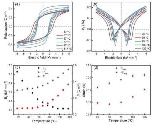
Fig. 5 (a) Polarization-electric field (P-E) and (b) strain-electric field (S-E) loops of 0.7BiFeO<sub>3</sub>-0.3Ba( $Ti_{0.995}Nb_{0.005}$ )O<sub>3</sub> ceramics measured at different temperatures. The temperature dependence of coercive field  $(E_c)$ , maximum  $(P_{max})$  and remanent  $(P_r)$  polarization obtained from P-E loops, and maximum strain ( $S_{max}$ ) and negative strain ( $-S_{neg}$ ) are summarised in (c) and (d) respectively.
