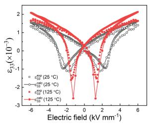
**Fig. 9** Comparison of longitudinal strain–electric field relationships determined by calculation from high resolution X-ray diffraction data (calc) and macroscopic strain–electric field (exp) measurements.
