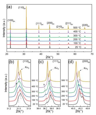
Fig. 1 (a) In situ XRD patterns of unpoled 0.5 mol% Nb-doped 0.7BF-0.3BT ceramics during heating. Details of the  $\{110\}_{pc}$ ,  $\{111\}_{pc}$  and  $\{200\}_{pc}$  peak profiles are shown in (b), (c) and (d) respectively. Arrow labels indicate the enhanced peak splitting of  $\{110\}_{pc}$  and  $\{111\}_{pc}$ , together with a gradual peak shift to lower angles due to thermal expansion, with increasing temperature
