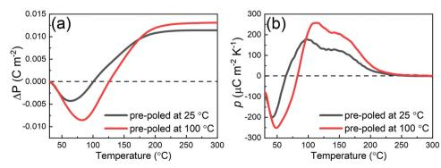
Fig. 6 Temperature-dependent changes in (a) remanent polarization, ΔP, and (b) pyroelectric coefficient, p, of 0.5 mol% Nb-doped 0.7BF-0.3BT prepoled at 25 and 100 °C.
