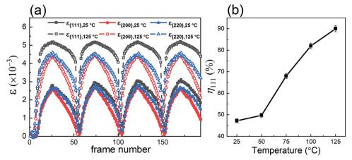
Fig. 8 (a) Influence of the applied electric field on effective lattice strains  $\varepsilon_{33}$  of Nb-doped 0.7BF-0.3BT ceramics for  $\{111\}_{DC}$ ,  $\{200\}_{DC}$  and  $\{220\}_{DC}$  at 25 and 125 °C. (b) Evaluated domain switching fraction,  $\eta$ , of (111) reflections, measured at various temperatures for the maximum field level.
