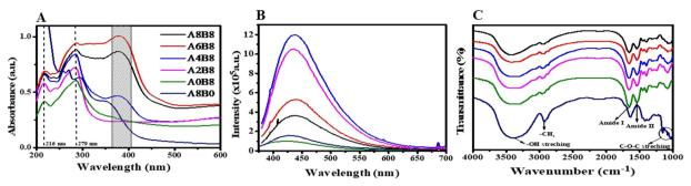
Fig. 3 Optical characterization of the lyophilized hydrogels. (A) UV-Vis absorbance spectra, (B) photoluminescence spectra, and (C) FTIR spectra, confirming the presence of the protein backbone, i.e., amide bonds.
