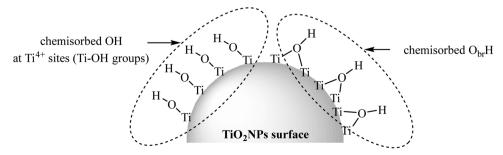
Fig. 1 Two different OH groups of the TiO<sub>2</sub>NP surface. Adapted with permission from ref. 20. Copyright 2014 American Chemical Society.
