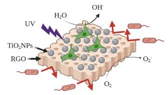
Fig. 7 The graphene oxide/titanium dioxide (RGO@TiO<sub>2</sub>) nanohybrid as a filler to investigate their synergistic effects on electrospun regenerated silk fibroin (RSF) mats. Adapted with permission from ref. 280. Copyright 2021 Elsevier.
