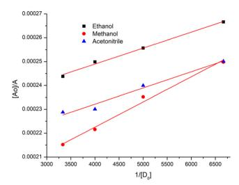
Fig. 3 Benesi-Hildebrand plots of CL, [A<sub>0</sub>]/A vs. 1/[D]<sub>0</sub>, in ethanol, methanol and acetonitrile at room temperature.
