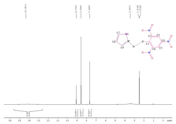
Fig. 1 <sup>1</sup>H NMR of the synthesized charge transfer complex (CL) of PYZ and TNP
