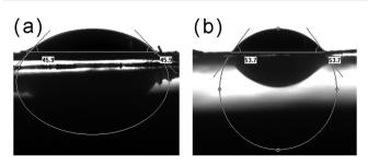
Fig. 4 Water contact angle of (a) Fe<sub>3</sub>O<sub>4</sub>@MOF and (b) ILs/Fe<sub>3</sub>O<sub>4</sub>@MOF
