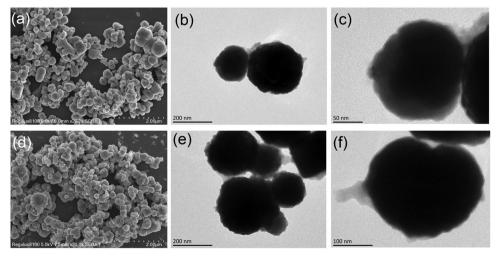
Fig. 3 SEM images of (a)  $Fe_3O_4@MOF$  and (d)  $ILs/Fe_3O_4@MOF$ . TEM images of (b and c)  $Fe_3O_4@MOF$  and (e and f)  $ILs/Fe_3O_4@MOF$ .
