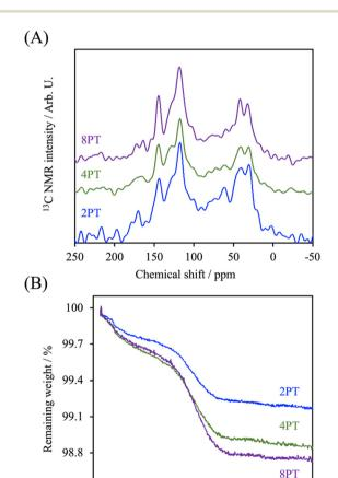
Fig. 2 (A) <sup>13</sup>C ssNMR spectra and (B) TGA curve of PDA-β-TCP synthesized at different concentrations of the DA precursor.
