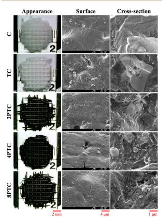
Fig. 4 Digital photographs and SEM micrographs of PCL and different β-TCP/PCL, composite scaffolds
