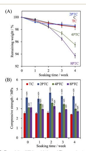
Fig. 6 The evolution of (A) the weight loss and (B) compressive strength of PCL, β-TCP/PCL, and PDA-β-TCP/PCL scaffolds after being immersed in SBF for different periods
