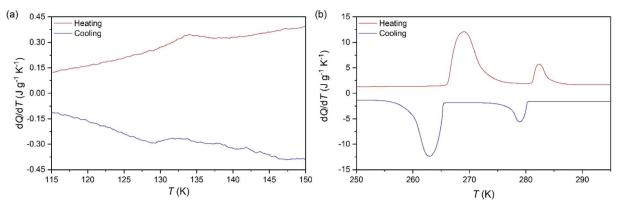
Fig. 1 VT-DSC curves for the [DBA][BF<sub>4</sub>] compound in the (a) lower- and (b) higher-temperature ranges.
