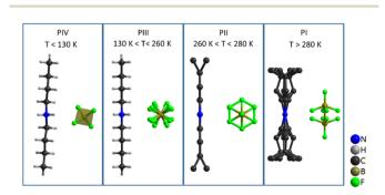
Fig. 9 Scheme of the molecular configuration of ions for the different phases of [DBA][BF<sub>4</sub>].
