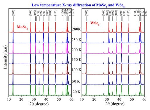
Fig. 1 The temperature dependence of XRD patterns of MoSe<sub>2</sub> (ICDD JCPDS-PDF 04-004-8782) and WSe<sub>2</sub> (ICDD JCPDS-PDF 00-038-1388). All the peaks are indexed using hexagonal symmetry with space group P63/mmc.
