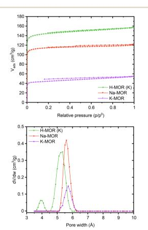
Fig. 5 Ar physisorption isotherms (top) and pore size distributions (bottom) obtained at 87K for a select number of samples (Na-MOR, K-MOR, H-MOR (K)).
