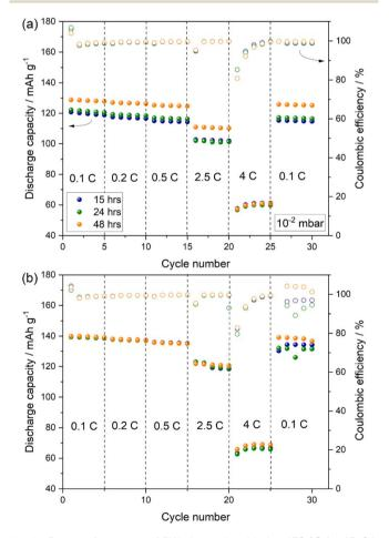
Fig. 9 Rate performance of PW electrodes dried at 170 °C for 15, 24, and 48 hours using a dynamic vacuum of  $10^{-2}$  (a) and  $10^{-3}$  mbar (b). Test conducted at 25 °C using 1 M NaPF<sub>6</sub> in diglyme electrolyte within the 2.0–4.0 V range. (1C = 140 mA g<sup>-1</sup>).
