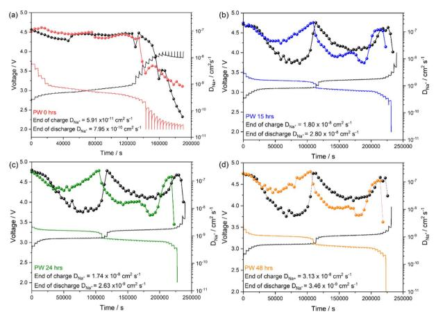
Fig. 10 GITT curves and corresponding calculated  $D_{\text{Na}^+}$  upon sodiation/de-sodiation for (a) undried (b) 15 hours, (c) 24 hours and (d) 48 hours PW electrodes dried at 170 °C under a dynamic vacuum of  $10^{-3}$  mbar.
