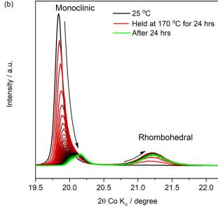
Fig. 4 In situ XRD measurement as a function of temperature on pristine PW-based composite electrodes. Test conducted in reflection mode (a) from room temperature (25 °C up to 200 °C, heating rate: 5 ° C min $^{-1}$ ). (b) From room temperature up to 170 °C with holding step for 24 hours. Both tests conducted under dynamic vacuum (10mbar).
