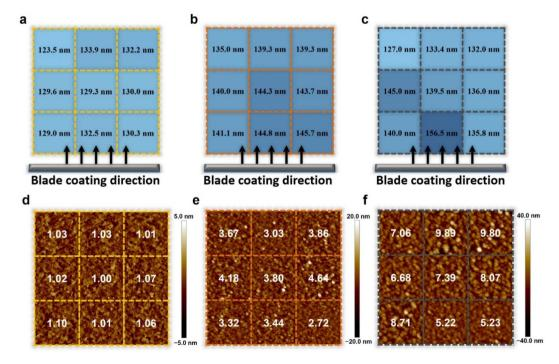
Fig. 4 Thickness and 2D height images of active layers from AFM for (a and d) PM6:L8-i-EB, (b and e) PM6:L8-i-EH, and (c and f) PM6:L8-i-BO with the RMS values of surface roughness on 5 cm  $\times$  5 cm substrates.
