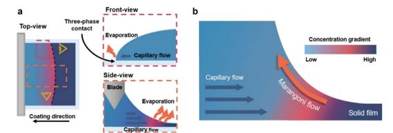
Fig. 2 (a) Schematic illustrations of non-uniform evaporation in the blade coating process in the top-view, side-view, and front-view. (b) Schematic illustration of two dominant convective flows: the capillary flow and the Marangoni flow in the side-view of the blade-coating process
