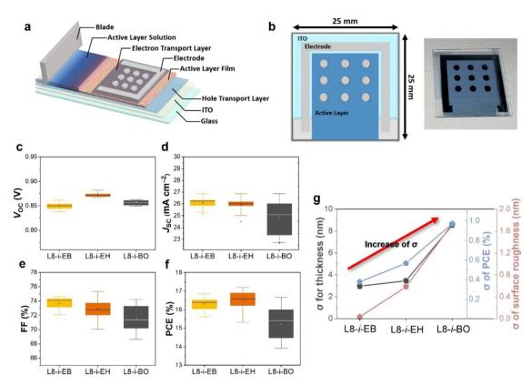
Fig. 5 (a) The schematic illustration of device fabrication via the blade-coating process with device configuration. (b) The illustration and picture of the 2.5 cm  $\times$  2.5 cm device. Distribution of (c)  $V_{OC}$ , (d)  $J_{SC}$ , (e) FF, and (f) PCE for L8-i-EB, L8-i-EH, and L8-i-BO based 9 devices on 2.5 cm  $\times$ 2.5 cm substrate. (g) The values of standard deviation for thickness, surface roughness of active layers, and PCEs based on PM6:L8-i-EB, PM6:L8i-EH, and PM6:L8-i-BO.
