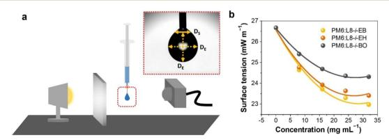
Fig. 3 (a) Illustration of the experimental setup of the pendant drop method and an image of a hanging droplet. (b) Surface tension of three NFAdissolved solutions depending on concentration.
