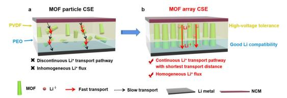
Fig. 2 Schematic illustrations of the Li<sup>+</sup> transport behaviors in (a) the MOF particle CSE and (b) MOF array CSE. The discrete MOF particles in the MOF particle CSE result in a discontinuous Li<sup>+</sup> transport pathway with an inhomogeneous Li<sup>+</sup> flux. Meanwhile, the MOF array CSE not only offers a continuous Li<sup>+</sup> transport pathway with the shortest transport distance between the cathode and anode, but also contributes to the homogeneous Li<sup>+</sup> flux.
