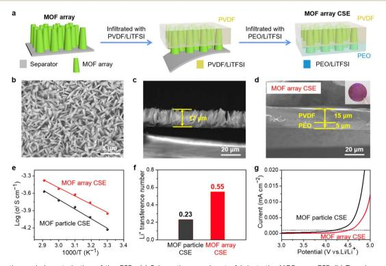
Fig. 3 Preparation and characterization of the CSEs. (a) Schematic procedure to fabricate the MOF array CSE. (b) Top view and (c) cross-sectional view SEM images of the MOF array grown on the separator. (d) Cross-sectional view of the MOF array CSE with bilayer polymer electrolytes. (e) Temperature-dependent ionic conductivities, (f) Li<sup>+</sup> transference numbers, and (g) oxidative stabilities of the MOF particle CSE and MOF array CSE.
