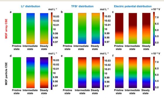
Fig. 5 COMSOL simulation results. The Li $^+$ , TFSI $^-$ , and electric potential distribution in (a–c) the MOF array CSE and (d–f) MOF particle CSE at pristine, intermediate, and steady states during Li $^+$  deposition at a current density of 0.2 mA cm $^{-2}$ .
