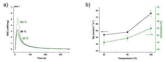
Fig. 2 (a) Photo-DSC of the PT-30 formulation at 80-100 °C,  $2 \times 900$  s, 320-500 nm, 60 mW cm<sup>-2</sup>. (b) Temperature dependence of rate of polymerization ( $R_p$  black) and conversion of the cyanate ester groups (green).
