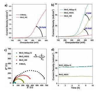
Fig. 2 (a) Polarization curves of  $\delta$ -MnO<sub>2</sub> and MnO<sub>x</sub>-NS. (b) Polarization curves of MnO<sub>x</sub>-NS, MnO<sub>x</sub>-NS/G, and MnO<sub>x</sub>-NS/py-G. (c) Nyquist diagrams of  $\delta$ -MnO<sub>2</sub>, MnO<sub>x</sub>-NS, MnO<sub>x</sub>-NS/G, and MnO<sub>x</sub>-NS/py-G. (d) Chronoamperometry curve of MnO<sub>x</sub>-NS/G and MnO<sub>x</sub>-NS/py-G at a 450 mV overpotential.
