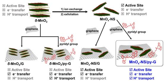
Scheme 2 Schematic illustration of the synthetic procedure of MnO<sub>2</sub>-NS/G, MnO<sub>2</sub>-NS/py-G, δ-MnO<sub>2</sub>/G, and δ-MnO<sub>2</sub>/py-G.
