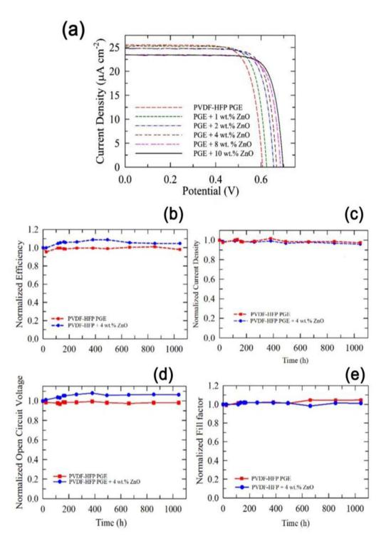
Fig. 4 (a) J-V curves of the QS-DSSCs using PVDF-HFP PGEs with and without various concentrations of ZnO nanofillers. (b) Normalized efficiency, (c)  $J_{sc}$ , (d)  $V_{oc}$ , and (e) FF of the QS-DSSC with and without 4 wt% ZnO nanofillers under continuous light illumination of 200 lx at 35 °C. (Reprinted from ref. 47 with permission from American Chemical Society).
