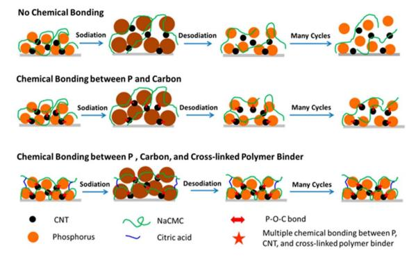
Fig. 18 Schematic illustration of structure evolution of phosphorus-base anode during cycling reproduced form ref. 134 with the permission from American Chemical Society.
