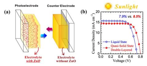
Fig. 5 (a) Schematic illustration of a DSSC featuring a "modified double-layered" electrolyte architecture. (b) Photovoltaic J-V curves related to the N719 DSSCs using modified double-layered electrolytes (under 1 sun). (Reprinted from ref. 48 with permission from Elsevier).
