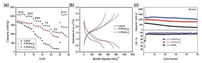
Fig. 15 (a) Rate characteristics of P-PPy/Fe $_3O_4$ , C-PPy/Fe $_3O_4$ , and control samples. (b) Charge/discharge profiles of P-PPy/Fe $_3O_4$ , C-PPy/Fe $_3O_4$ , and control samples at 1C rate. (c) Cyclic characteristics and corresponding coulombic efficiency of P-PPy/Fe<sub>3</sub>O<sub>4</sub>, C-PPy/Fe<sub>3</sub>O<sub>4</sub>, and control samples at a current density of  $100 \text{ mA g}^{-1}$  reproduced from ref. 117 with permission from Wiley-VCH.
