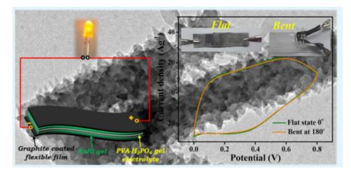
Fig. 22 Flexible supercapacitor assembled with MoS₂ quantum dot (QD)/PANI hydrogel electrodes and PVA/H₂SO₄ gel electrolyte, reproduced with permission from ref. 179 with permission from the American Chemical Society.
