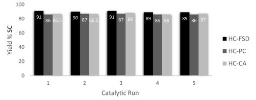
Fig. 9 Recycling catalytic test for the coupling of SO and  $CO_2$  catalyzed by HC-FSD, HC-PC and HC-CA. Reaction conditions: 0.875 mmol SO (100  $\mu$ L), autoclave, p ( $CO_2$ ) 3 bar, catalyst loading 10 wt%, temperature 70 °C, 7 h. Isolated yields are given, after purification of the reaction crude by flash column chromatography. Yield of SC was the average after two runs. Selectivity was > 99% for all catalytic runs.
