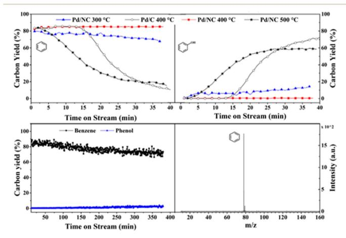
Fig. 15 Time-onstream for Pd/C and Pd/NC at 400 °C and 500 °C (top). Catalyst stability for guaiacol HDO over Pd/NC (bottom). Reproduced from ref. 80 with permission from Elsevier, copyright 2021.
