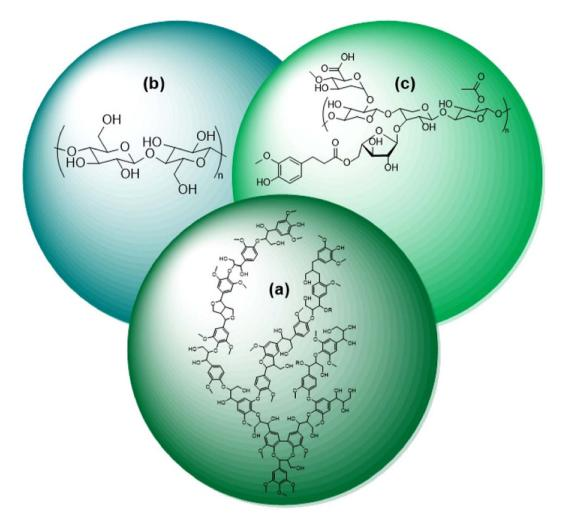
Fig. 1 Substructures of biomass: (a) lignin, (b) cellulose, and (c) hemicellulose.
