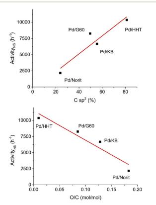
Fig. 13 Correlation between catalytic activity and graphitization order (top) and correlation between catalytic activity and oxygen functionalization (bottom). Reproduced from ref. 78 with permission from ACS, copyright 2019
