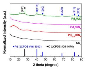
Fig. 24 XRD patterns of different Pd ratios on activated carbon and Ndoped carbon supports. Reproduced from ref. 112 with permission from American Association for the Advancement of Science, copyright 2020
