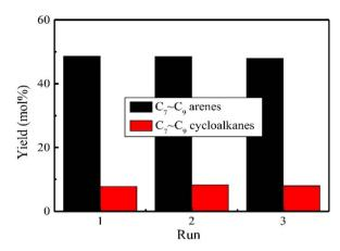
Fig. 11 Products distribution in three successive runs during the HDO of enzymatic lignin over Ru/L1-Nb<sub>2</sub>O<sub>5</sub> catalyst. Reproduced from ref. 74 with permission from Elsevier, copyright 2019.
