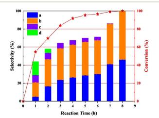
Fig. 14 Time-onstream performance of Pd/CN<sub>x</sub> for the conversion of veratryl alcohol. Reproduced from ref. 79 with permission from Elsevier, copyright 2021.
