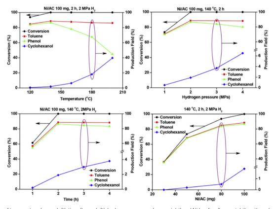
Fig. 6 Effects of temperature (upper left), time (lower left), hydrogen pressure (upper right) and Ni loading (lower right) on the selective cleavage of BPE. Reproduced from ref. 54 with permission from J. Energy Inst., copyright 2019.
