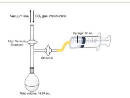
Fig. 4 Outline of the experimental setup for the estimation of the amount of  $CO_2$  in the gas phase captured in a sample solution.
