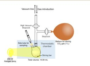
Fig. 5 Outline of the experimental setup of the isobaric system utilized for direct capture of CO<sub>2</sub> gas.
