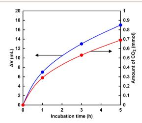
Fig. 6 Time dependence of the volume change ( $\Delta V$ ) of the syringe of the experimental apparatus ( ) and calculating the amount of CO<sub>2</sub> from the volume change of the syringe (
