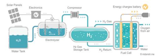
Fig. 1 A typical green hydrogen fuel cell representation.
