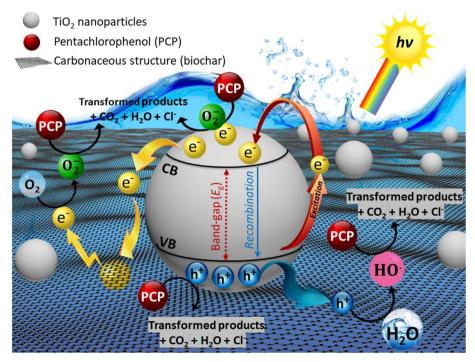
Possible reaction mechanisms of CGBT for the photocatalytic degradation.
