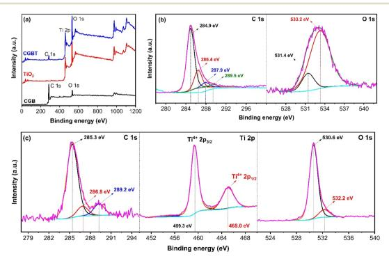
Fig. 4 (a) XPS full-scan spectra of the synthesized materials. (b) High-resolution XPS C 1s and O 1s spectra of coffee ground-biochar (CGB). (c) High-resolution XPS C 1s, Ti 2p and O 1s spectra of CGBT nanocomposites.
