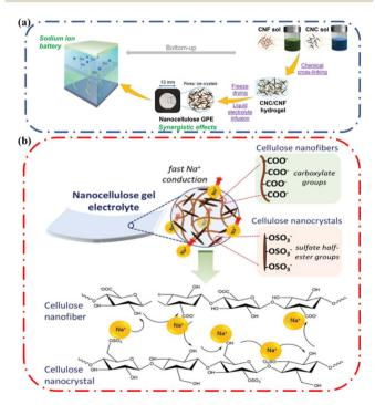
Fig. 10 (a) Schematic representation of the nanocellulose gel electrolyte fabrication. (b) Schematic illustration of the proposed  $\mathrm{Na}^+$  conduction mechanism across the nanocellulose Gel Polymer Electrolytes (GPE). Reprinted with permission from Mittal *et al.*<sup>62</sup> Copyright 2022 Wiley.
