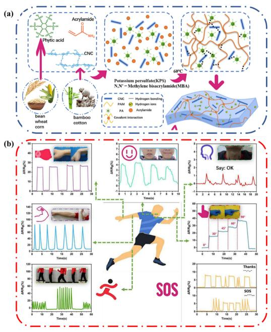
Fig. 16 (a) Illustration showing the formation of the biomass-reinforced hydrogels (b) variation of  $\Delta R/R_0$  of the hydrogel at room temperature during palm movement, smiling and talking, arm movement, finger bending, walking, and running. Information delivery using the hydrogel as a strain sensor *via* Morse codes. Reprinted with permission from Wang *et al.*<sup>75</sup> Copyright 2022 Elsevier.
