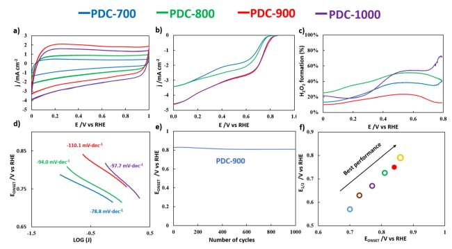
Fig. 4 (a) Cyclic voltammetry in 0.1 M KOH, N<sub>2</sub>-saturated solution at 50 mV s<sup>-1</sup>; (b) linear sweep voltammetry in 0.1 M KOH, O<sub>2</sub>-saturated solution at 1600 rpm; (c) H<sub>2</sub>O<sub>2</sub> formation; (d) Tafel slopes of all PDC-T materials; (e) stability of PDC-900 under continuous LSV cycling; (f) literature comparison of the ORR performance of other P-doped materials (unfilled circles) to PCD-900 (red solid circle)
