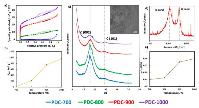
Fig. 2 (a)  $N_2$  adsorption (full symbols) – desorption (empty symbols) isotherms of the PDC-T series; (b) plot of  $A_{\rm BET}$  obtained from  $N_2$  adsorption isotherms; (c) XRD patterns of the PDC-T series and TEM image of PDC-900 (inset); (d) Raman spectra of PDC-900; and (e) plot of  $I_D/I_G$  ratio obtained from Raman spectra.
