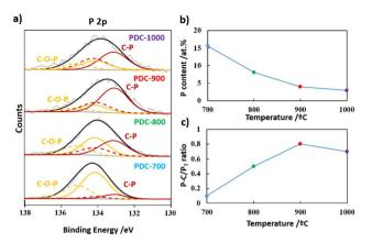
Fig. 3 (a) P 2p XPS spectra, (b) P content, and (c)  $P-C/P_T$  ratio of the PDC-T series.
