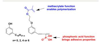
Fig. 12 Chemical structure of cardanol and phosphonated cardanol methacrylate.
