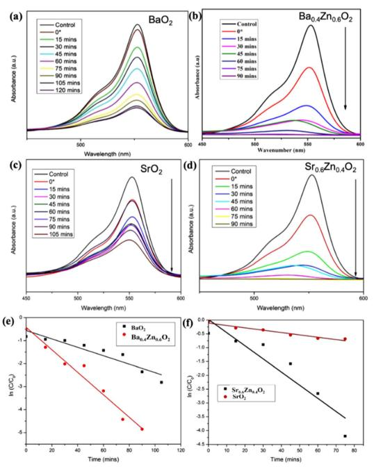
Fig. 9 The photocatalytic degradation efficiency of RhB by (a)  $BaO_2$ , (b)  $Ba_{0.4}Zn_{0.6}O_2$  (c)  $SrO_2$  and (d)  $Sr_{0.6}Zn_{0.4}O_2$  photocatalysts under direct sunlight. First-order-kinetics plots of RhB degradation using (e)  $BaO_2$  and  $Ba_{0.4}Zn_{0.6}O_2$  and (f)  $SrO_2$ .
