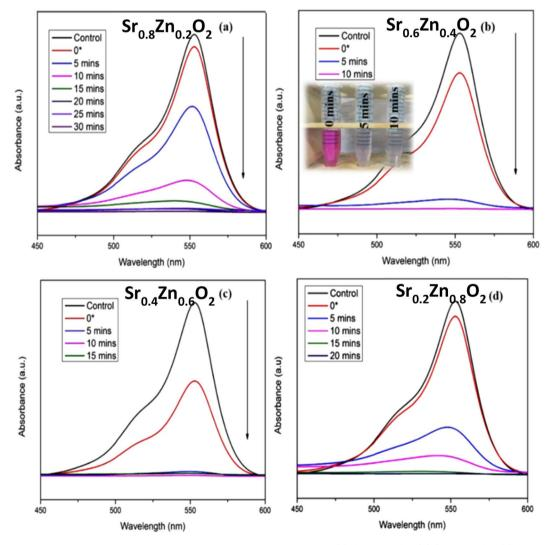
Fig. 8 Influence of Zn doping on the photocatalytic degradation of RhB using (a)  $Sr_{0.8}Zn_{0.2}O_2$ , (b)  $Sr_{0.6}Zn_{0.4}O_2$ , (c)  $Sr_{0.4}Zn_{0.6}O_2$ , and (d) Sr<sub>0.2</sub>Zn<sub>0.8</sub>O<sub>2</sub> photocatalysts under UV light irradiation.
