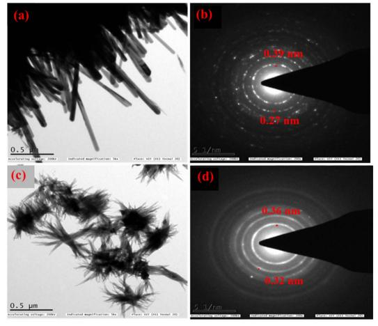
Fig. 4 HRTEM and SAED images of (a and b)  $Ba_{0.4}Zn_{0.6}O_2$  and (c and d)  $Sr_{0.6}Zn_{0.4}O_2$ .
