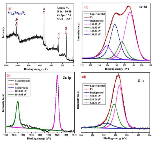
Fig. 6 XPS spectra, (a) survey scan of (b) Sr 3d, (c) Zn 2p and (d) O 1s of Sr<sub>0.6</sub>Zn<sub>0.4</sub>O<sub>2</sub>.
