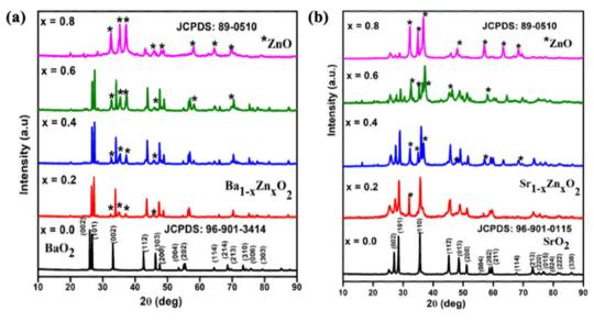
Fig. 1 XRD patterns of (a)  $Ba_{1-x}Zn_xO_2$  and (b)  $Sr_{1-x}Zn_xO_2$ , x = 0.2, 0.4, 0.6, 0.8
