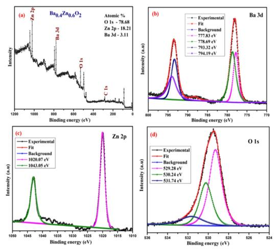
Fig. 5 XPS spectra, (a) survey scan of (b) Ba 3d, (c) Zn 2p and (d) O 1s of Ba<sub>0.4</sub>Zn<sub>0.6</sub>O<sub>2</sub>.
