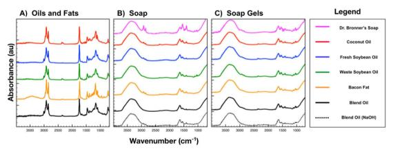
Fig. 4 IR spectra of (A) fresh and waste oils and fats, (B) saponified mixtures of fresh and waste oils and fats, and soap and (C) soap gels from fresh and waste oils and fats, and commercial soap. Oils are saponified with potassium hydroxide (KOH) unless otherwise noted.
