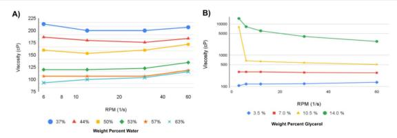
Fig. 3 Graphs showing (A) the changing viscosity of bacon fat soap dilutions with water and (B) the non-Newtonian behaviors of soap-glycerol mixtures. Varying concentrations can help tailor material properties of the soaps
