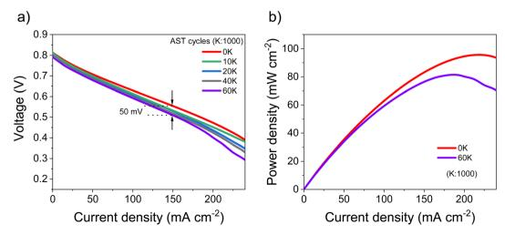
Fig. 9 (a) Fuel cell polarization curves at various cycles of operation under AST, (b) comparison of power density between the first cycle (0 K) and final cycle (60 K). Performance was monitored in the voltage range of 0.5-0.6 V at the current density of 150 mA cm<sup>-2</sup>.
