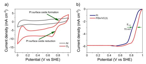
Fig. 6 ORR activity of PtSn/VC(3), (a) CV at scan rate 50 mV s<sup>-1</sup> @ 1600 rpm in 0.1 M aqueous HClO<sub>4</sub> under saturated Ar and O<sub>2</sub>, (b) LSV comparison between PtSn/VC(3) and Pt/VC at the scan rate of 10 mV s<sup>-1</sup> @ 1600 rpm under saturated  $O_2$ . Catalyst loading was 50  $\mu$ g cm<sup>-2</sup>.
