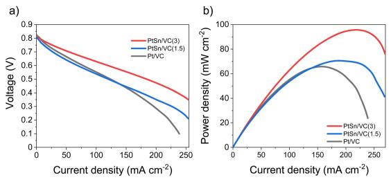
Fig. 8 Performance of PtSn/VC(3), PtSn/VC(1.5) and Pt/VC in a self-breathing PEMFC, (a) current density vs. voltage, (b) current density vs. power density. The catalyst loading at the active area of both the anode and cathode was  $0.8 \text{ mg cm}^{-2}$ . The same catalyst was loaded at both side of the MEA. The  $H_2$  flow rate was 10 mL min<sup>-1</sup>.
