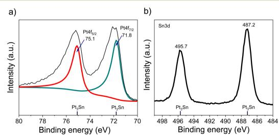
Fig. 4 XPS spectra of PtSn/VC(3), (a) Pt 4f, (b) Sn 3d.
