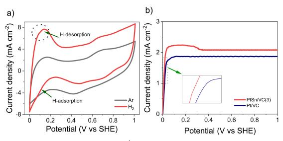
Fig. 5 HOR activity of PtSn/VC(3), (a) CV at scan rate 50 mV s<sup>-1</sup> @ 1600 rpm in 0.1 M aqueous HClO<sub>4</sub> under saturated Ar and H<sub>2</sub>, (b) LSV comparison between PtSn/VC(3) and Pt/VC at the scan rate of 10 mV s<sup>-1</sup> @ 1600 rpm under saturated H<sub>2</sub>. Catalyst loading was 50 µg cm<sup>-2</sup>.
