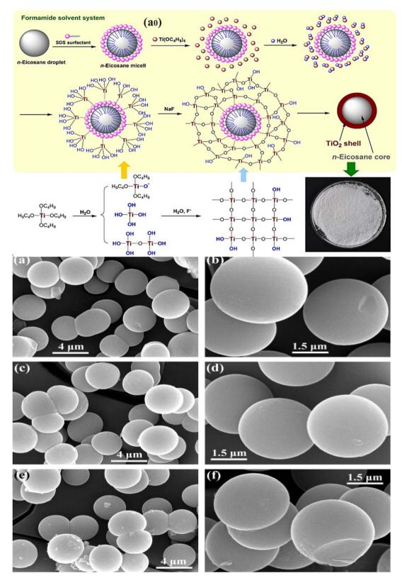
Fig. 15 (a0) Schematic illustration of the fabrication of the n-eicosane microcapsule TiO $_2$  shell, SEM images of the n-eicosane microcapsule (a and b) produced with a weight ratio of 60/40 n-eicosane/TBT, (c and d) produced with a weight ratio of 50/50 n-eicosane/TBT, and (e and f) produced with a weight ratio of 40/60 n-eicosane/TBT. $^{129}$  Reproduced with permission from ref. 129 Copyright 2015 Elsevier.
