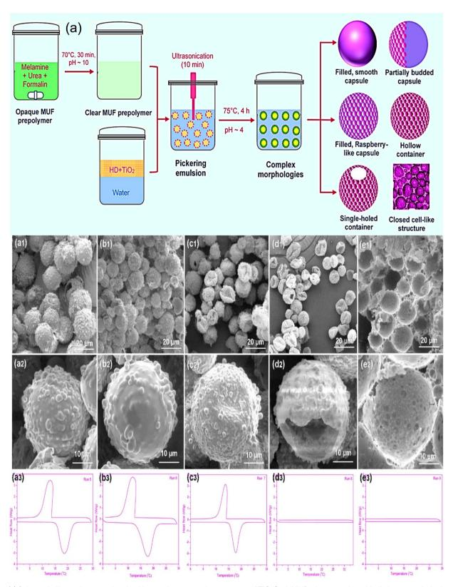
Fig. 5 (a) Schematic illustration steps involved in creating a complex structure of  $TiO_2$ /polyMUF microcapsules with distinct morphologies, DSC thermograms, and SEM images of the microcapsules at different core-to-shell ratios, (a1–a3) core-to-shell ratio of 1:2, (b1–b3) core-to-shell ratio of 1:1, (c1–c3) core-to-shell ratio of 2:1. A ratio of 1:0.5, (d1–d3) core-to-shell ratio of 1:5:1, and (e1–e3) core-to-shell ratio of 2:1. Reproduced with permission from ref. 141 Copyright ACS 2022.
