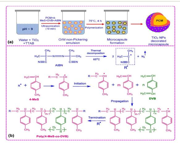
Fig. 7 (a) Schematic illustration for the creation of a crosslinked polystyrene-based shell decorated with  $TiO_2$  nanoparticles and (b) free radical polymerization for the creation of the poly(4-methylstyrene-co-divinylbenzene) shell.<sup>47</sup> Reproduced with permission from ref. 47. Copyright 2021 ACS.
