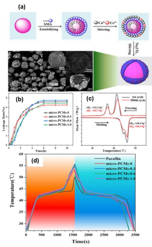
Fig. 19 (a) Schematic of synthesis for paraffin microcapsules composed of Ce<sup>3+</sup> dopped calcium carbonate with SEM images; (b) Leakage rate of paraffin microcapsules; (c) DSC curves of PCM microcapsules containing 0.6 wt% Ce<sup>3+</sup> with respect to calcium carbonate; (d) paraffin and paraffin microcapsules' temperature – time curves during the release processes (blue) and storage (red). <sup>177</sup> Reproduced with permission from ref. 177 Copyright 2019 ACS.
