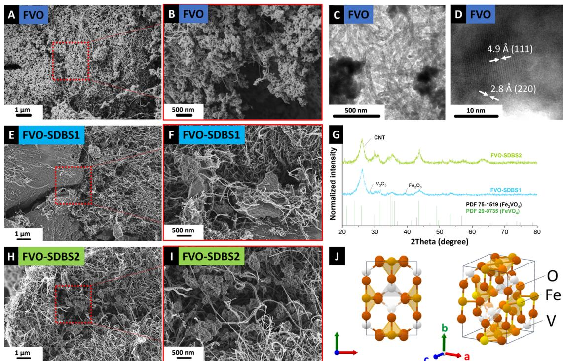
Fig. 3 (A) and (B) Scanning electron micrographs and (C) and (D) transmission electron micrographs of FeV grown *in situ* on CNT after oxidation, (E) and (F) scanning electron micrographs of FeV with SDBS added to hexacyanoferrate after oxidation, (G) X-ray diffractogram of FVO-SDBS1 and FVO-SDBS-2, (H) and (I) scanning electron micrographs of FeV with SDBS added to vanadyl sulfate after oxidation and (J) crystal structure of FeVO<sub>4</sub>.
