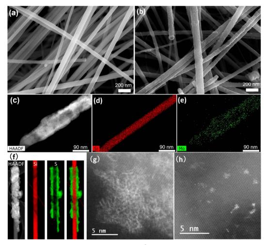
Fig. 4 SEM images of (a) 48 nm-SiNWs, (b) SiNW-MoS<sub>x</sub> with  $\Delta Q = 6$  mC cm<sup>-2</sup> (c) HAADF-STEM image of SiNW-MoS<sub>x</sub> and EDX mapping profile of (d) Si(K<sub>x</sub>) and (e) Mo(K<sub>x</sub>); (f) STEM-HAADF image and EELS mapping profile of element Si (L edge at 99 eV) and S (L edge at 165 eV); (g, h) High-resolution HAADF-STEM images of a-MoS<sub>x</sub>.
