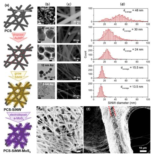
Fig. 2 Tuning SiNW diameter by the size of AuNPs: (a) scheme of the PCS-SiNW-MoS $_x$  photocathode fabrication. SEM and TEM images of the AuNPs of size 3-80 nm (b) and the subsequent SiNWs grown from them (c); (d) corresponding SiNW diameter histograms (>500 counts); SEM images of the PCS-SiNW (e) and close up view of a single carbon fiber (f). Red dotted lines highlight the diameter of the carbon fiber.
