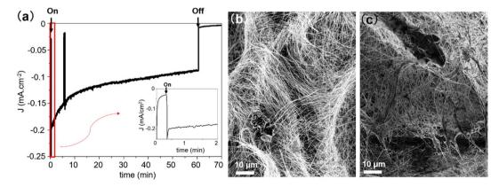
Fig. 7 (a) Chronoamperometry of PCS-SiNW-MoS $_{x}$  at -0.15 V vs. RHE in 0.5 M H $_{2}$ SO $_{4}$  under illumination (48 nm-SiNWs,  $\Delta Q_{MoS}_{\chi} = 6$  mC cm $^{-2}$ ) with N $_{2}$  bubbling. SEM images of the electrode before (b) and after (c) the stability test.
