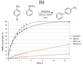
**Fig. 8** SEM image of the Pd/graphite catalyst after MW treatment in air for 5 min (a) and NMR monitoring of the Suzuki–Miyaura reaction of 1-bromo-4-nitrobenzene with phenylboronic acid in the presence of Pd/graphite catalysts MW-treated for different durations (b). Reproduced from ref. 68 with permission of American Chemical Society, copyright 2017.
