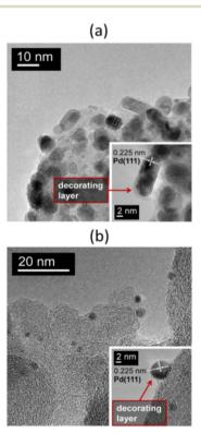
Fig. 6 TEM images at different magnifications of the 1% Pd/NGC catalysts prepared by impregnation of the carbon support with solutions of  $Pd_3(OAc)_6$  (a) and  $Pd_2(dba)_3$  (b) in chloroform followed by treatment in flowing hydrogen at 300 °C. In both cases, the Pd NPs are encapsulated by amorphous carbon formed during the high-temperature decomposition of these palladium complexes. Reproduced from ref. 47 with permission of Elsevier, copyright 2020.
