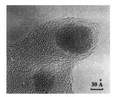
Fig. 7 TEM image of a Pd NP encapsulated in the carbon support by the "shrinkage-following-swelling" mechanism. This NP was formed via spontaneous reduction of aqueous  $H_2[PdCl_4]$  by the surface of the furnace NGC at 20 °C. Reproduced from ref. 32 with permission of CRC Press and Taylor & Francis Group, copyright 2003.
