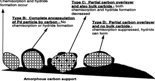
Fig. 5 Palladium NPs with various extents of encapsulation by carbon and bulk carbide formation. Reproduced from ref. 60 with permission of Elsevier, copyright 1998.
