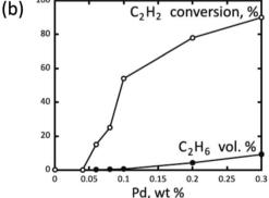
Fig. 4 Carbon nanostructures with different arrangements of graphene layers (a) and performance of Pd/pCNF catalysts with different palladium contents in the gas-phase hydrogenation of acetylene in its mixture with ethylene at 90 °C (b). (a) is reproduced from ref. 28 with permission of the Royal Society of Chemistry, copyright 2015, and (b) is reproduced from ref. 53 with permission of Elsevier, copyright 2012.
