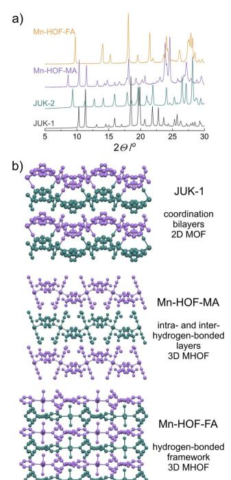
Fig. 2 Structural transformation between JUK-1 and Mn-HOFs. (a) PXRD patterns for JUK-1 and Mn-HOFs, compared with related JUK-2. (b) Stacked coordination bilayers in the initial JUK-1 (top), and the resulting: stacked hydrogen-bonded layers in Mn-HOF-MA (middle) and 3D hydrogen-bonded network in Mn-HOF-FA (bottom), all packing views along the c axes. The layers in JUK-1 and Mn-HOF-MA are stabilized by interlayer hydrogen bonds.
