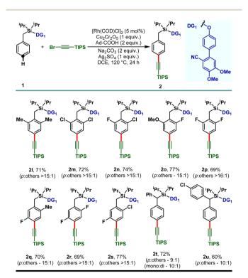
Scheme 3 Rh-catalyzed *para-*C-H alkynylation of di-substituted arenes.
