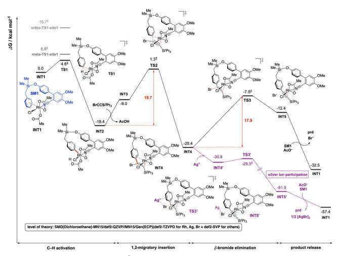
Fig. 1 Gibbs energy profile for the Rh-catalyzed C(sp<sup>2</sup>)-H alkynylation of arenes. DFT optimized key transition structures are shown in Fig. 2.
