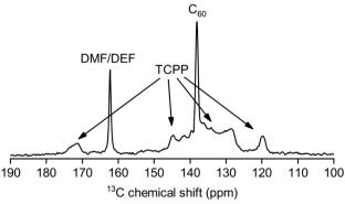
Fig. 4 (Up)  $^1$ H MAS NMR spectra for Cu<sub>0.1</sub>-PCN-223 and  $1.0C_{60}$ @Cu<sub>0.1</sub>-PCN-223 at 300 K. (Down)  $^{13}$ C MAS NMR spectrum of  $1.0C_{60}$ @Cu<sub>0.1</sub>-PCN-223 at 300 K. The signals from dimethylformamide (DMF), diethylformamide (DEF), H<sub>2</sub>TCPP linker and fullerene (C<sub>60</sub>) are indicated on the spectra.
