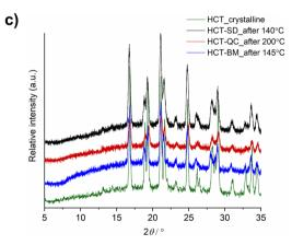
Fig. 2 (a) mDSC thermograms of HCT polyamorphs obtained by SD, QC and BM after a second heating cycle (total heat flow); (b) mDSC (total and reversing heat flow) and TGA of polyamorph I (obtained by SD) after the second heating cycle; (c) PXRD data of all HCT polyamorphs obtained after the recrystallization temperature.
