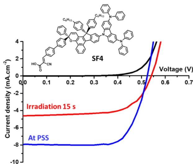
Fig. 4  $J$ - $V$  curves of a SF4-based opaque photochromic solar cell registered in the dark (black line), after 15 seconds under irradiation (red line) and at PSS reached after 300 seconds under continuous irradiation (blue line). Standard irradiation conditions were AM 1.5 G, 1000 W  $\times$  m<sup>-2</sup> at 25 °C.
